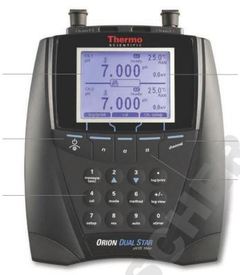
Selectable read modes include Auto-Read, On-Ready, At Timed Intervals, Continuous, Value Change in Measurement and Timed for a variety of measurement collection methods for different analytical methods
