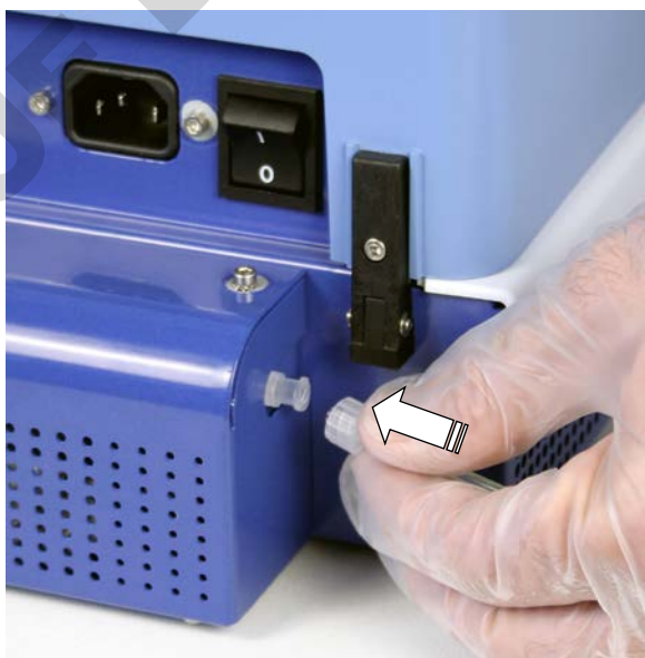
Figure 3–10. Connecting the hosing to the pressure/vacuum system
