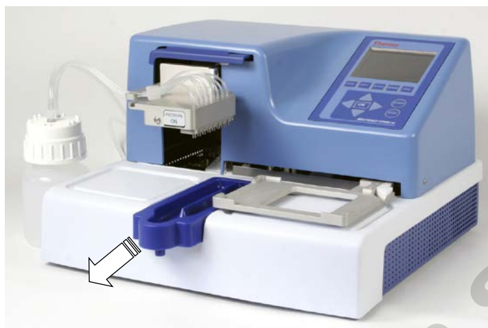
Figure 5–32. Unfastening the priming vessel
