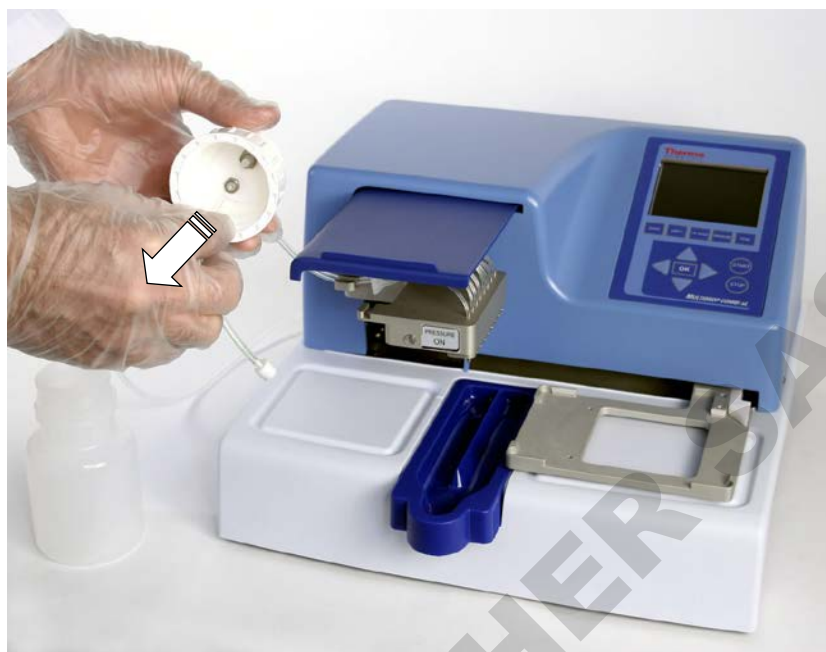
Figure 5–27. Removing the reagent filter with tube
