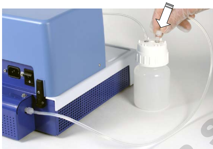
Figure 3-11. Connecting the hosing to the reagent reservoir
