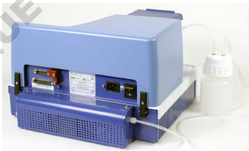
Figure 5–33. Transport lock storage location
