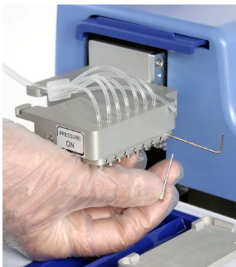
Figure 5–30. Replacing the dispensing valve
