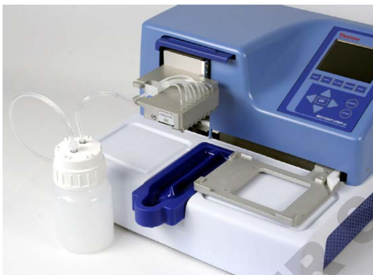
Figure 3–13. Reagent reservoir connected to the instrument
