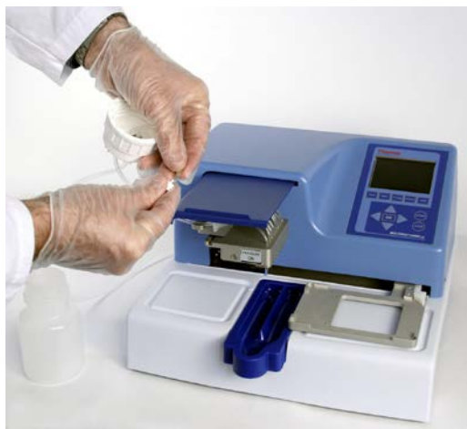
Figure 5–23. Removing the reagent filter
