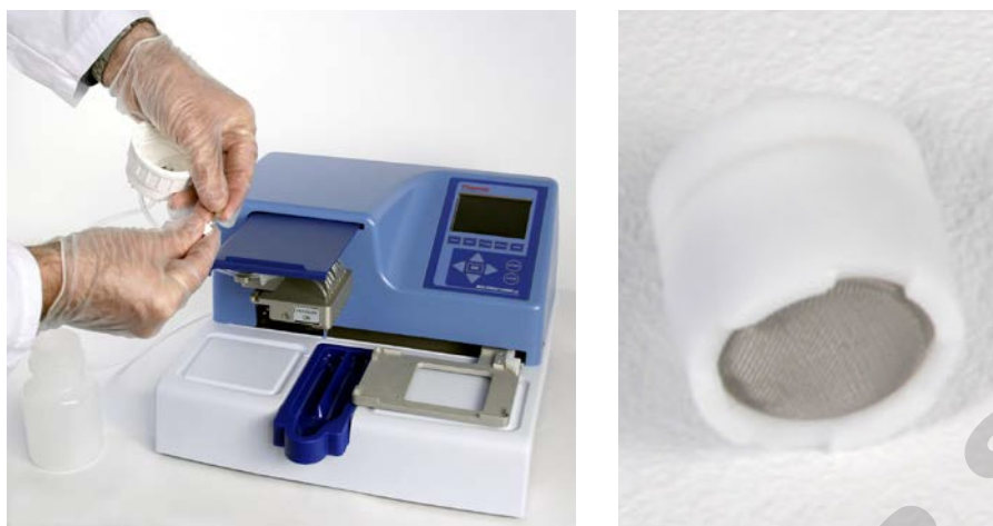
Figure 4-18. Removing the reagent filter
