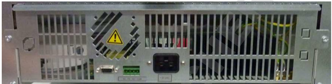
Figure 5-9 AC Power Supply Socket
