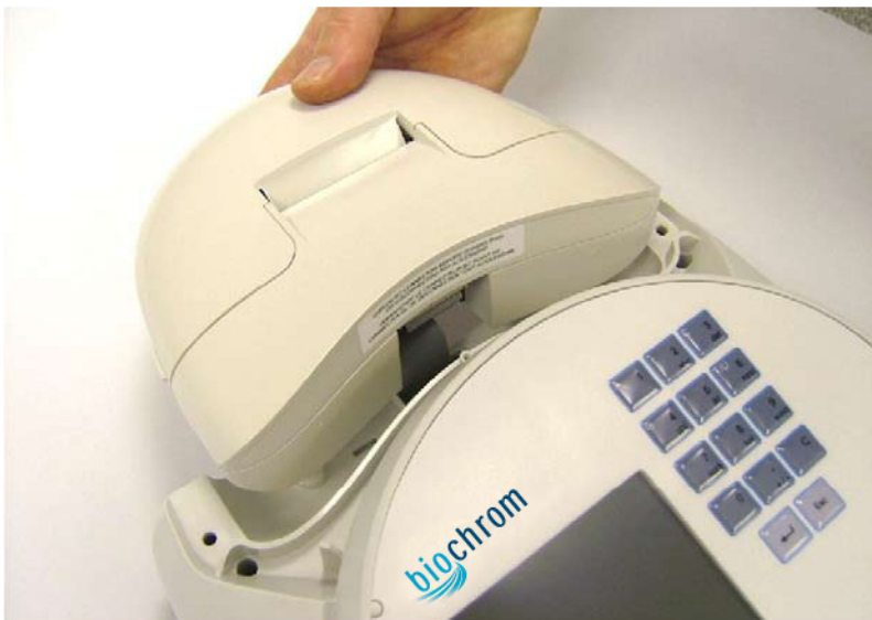
Figure: 15 Step 4. Lower the printer onto the locating bosses.
