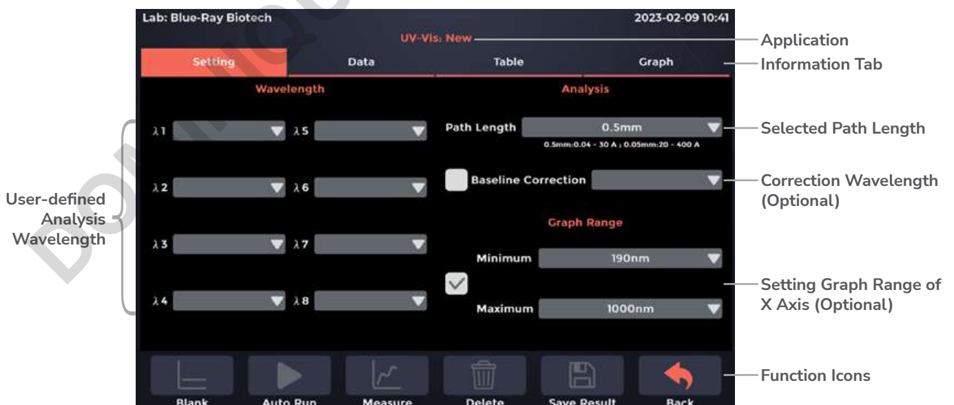
Figure 46. Setting Tab Page of UV-Vis Application
