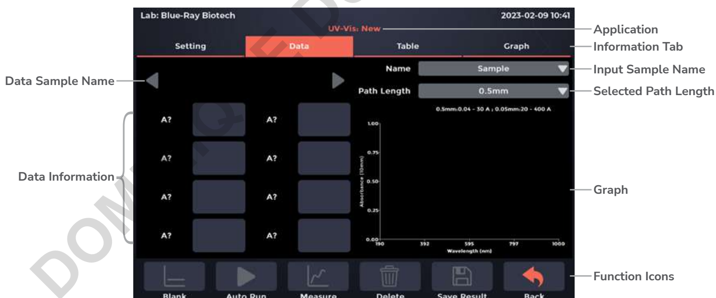
Figure 47. Data Tab Page of UV-Vis Application
