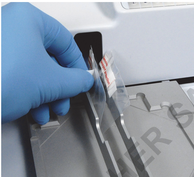
Figure 2–6. Transport lock and transport lock tag
