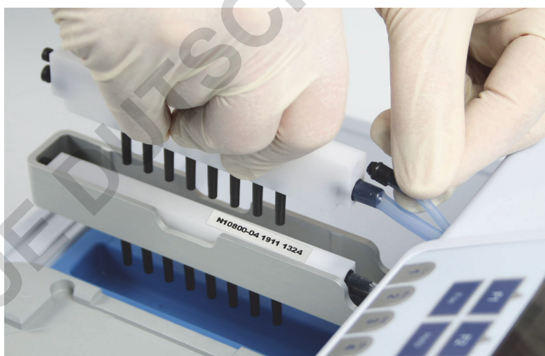
Figure 2–10. Fitting the wash heads to the connectors
