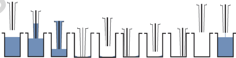
Figure 1-4. Principle of washing step (Sweep2)
