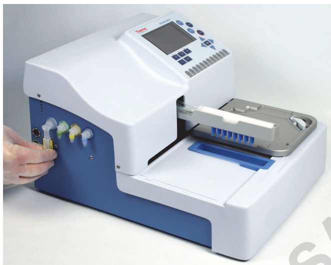
Figure 2–18. Connecting the liquid bottle tubing
