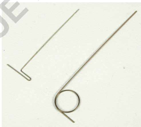
Figure 11–45. Thin and normal declogging tools
