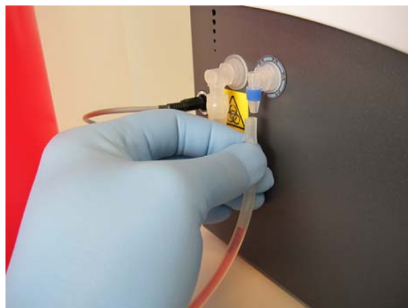
Figure 40. Manually priming a dry pump. Colored liquids are used for illustrative purposes.
