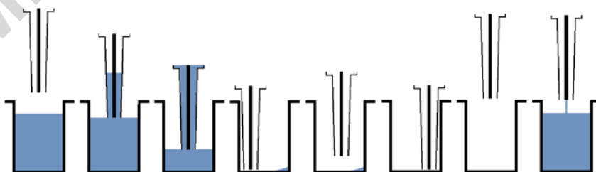
Figure 4. Principle of Wash step (Sweep2)
