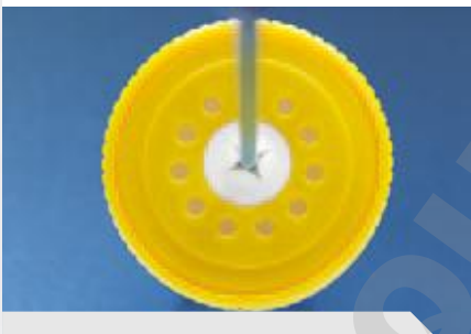
Septum made of Silicone
