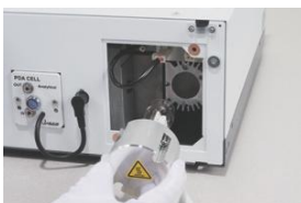
Front panel access for easy lamp replacement
