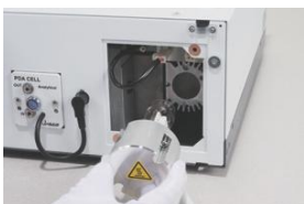
Front panel access for easy lamp replacement
