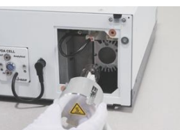
Front panel access for easy lamp replacement
