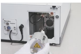
Front panel access for easy lamp replacement
