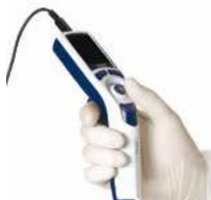
Figure 26: Operating the pipette while connected to E4-WPS Wall Power Supply
