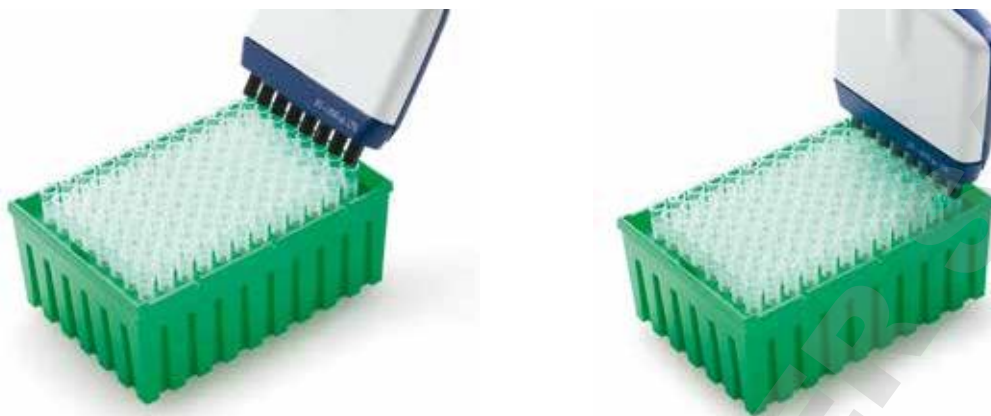
Figure 35: Mounting Racked LTS Tips
