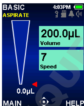
Figure 11: Basic Mode Aspirate Operation.
