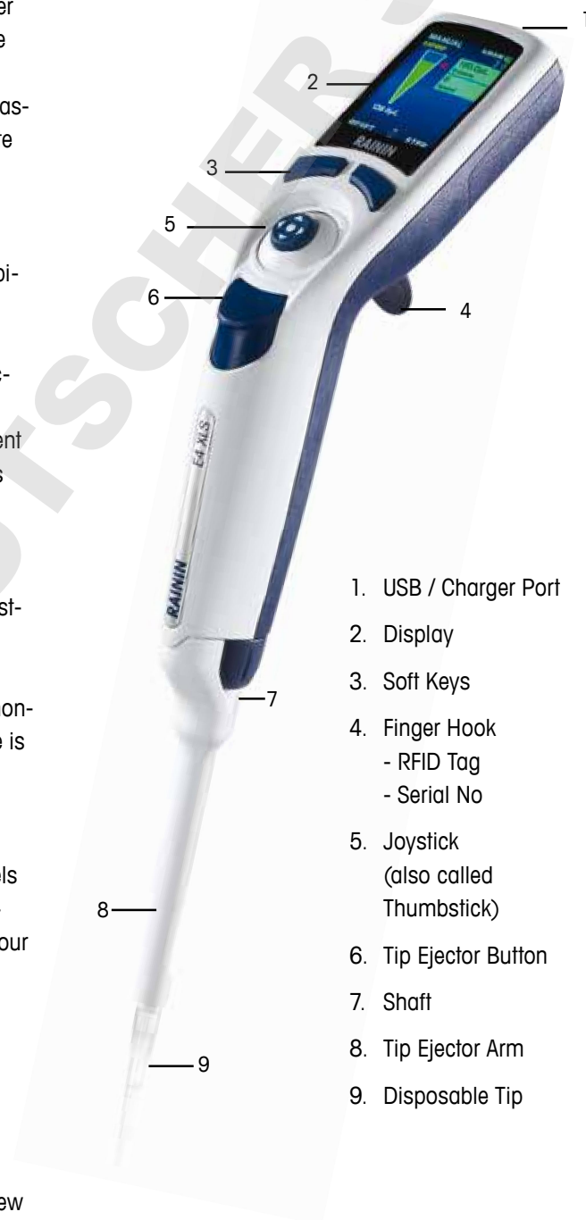
Figure 1: E4 XLS Single-channel Pipette
