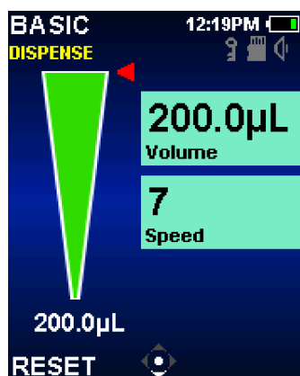
Figure 12: Basic Mode Dispense Operation.
