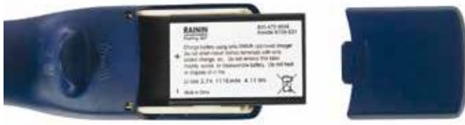
Figure 5: Installing the main battery
