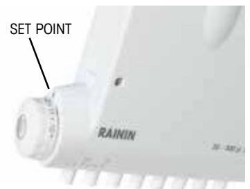
Figure 37: Limiter Set Point
