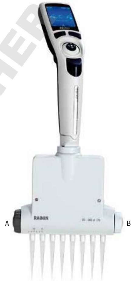
Figure 36: E4 XLS Adjustable Spacer A: SPACING ADJUSTMENT B: LIMITER
