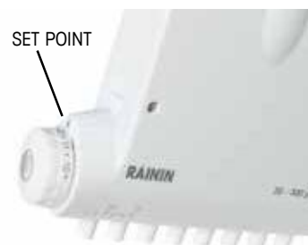
Figure 37: Limiter Set Point
