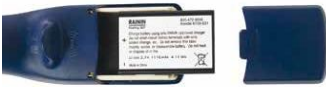
Figure 5: Installing the main battery
