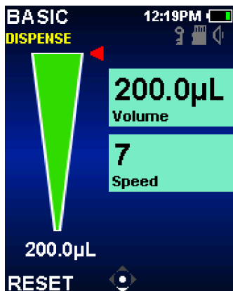
Figure 12: Basic Mode Dispense Operation.
