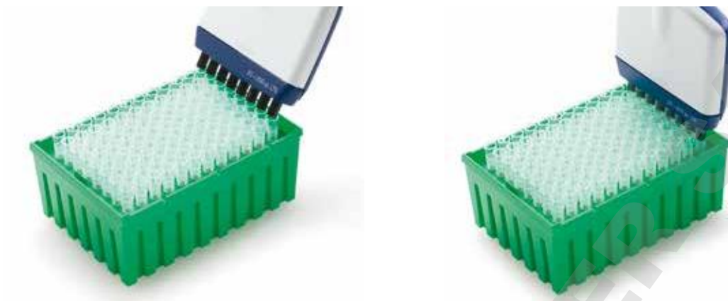
Figure 35: Mounting Racked LTS Tips
