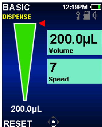
Figure 12: Basic Mode Dispense Operation.
