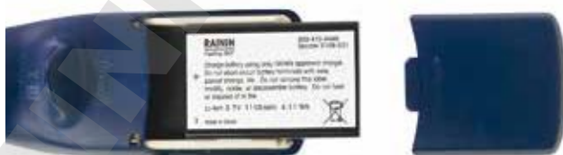
Figure 28: Replacing the Battery
