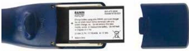
Figure 5: Installing the main battery
