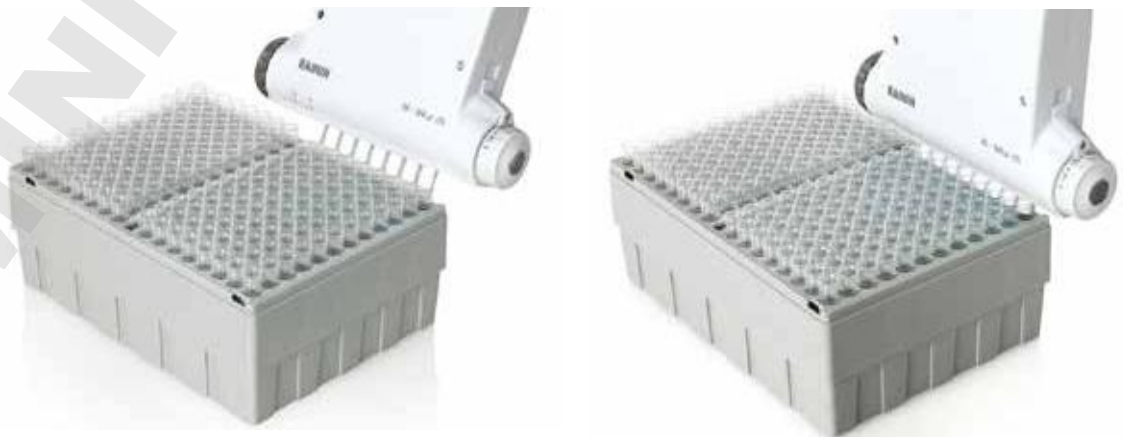
Figure 39: Mounting LTS Tips
