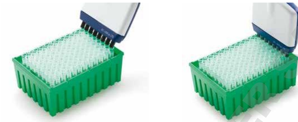
Figure 35: Mounting Racked LTS Tips
