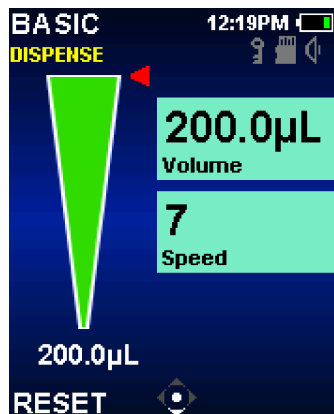
Figure 12: Basic Mode Dispense Operation.
