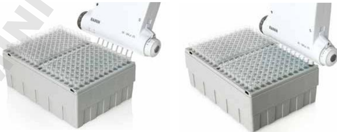
Figure 39: Mounting LTS Tips
