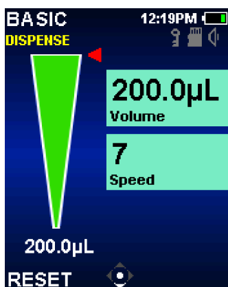
Figure 12: Basic Mode Dispense Operation.
