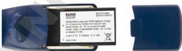
Figure 28: Replacing the Battery
