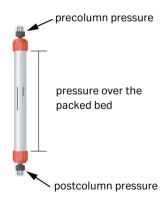
Fig 10. Precolumn and post-column measurements.
