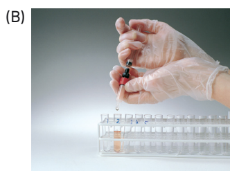
Fig 2. Using HiTrap IgM Purification HP with a syringe. (A) Prepare buffers and sample. Remove the top cap of the column and snap off the end. Wash and equilibrate. (B) Load the sample and begin collecting fractions. (C) Wash, elute and continue collecting fractions.
