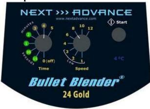
The figure above shows the Bullet Blender Gold set to run for 4 minutes at a speed of 8, after running for 2 minutes. To operate, press the "START" button. After 15 seconds, the LED light by the number 15 will light up. After 30 seconds, the second LED light by the number 30 will light up. And so on. At the settings shown above, after 4 minutes, the Bullet Blender Gold will stop.
