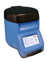
The Bullet Blender® enables you to homogenize, disrupt, or lyse up to 24 tissue or cell culture samples at a time. Load the samples into standard polypropylene tubes, then place them in the Bullet Blender homogenizer. The "bullets" in the instrument vigorously strike all of the tubes and homogenize your sample in minutes. The Bullet Blender Gold models keep samples at 4°C!
