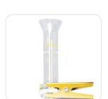
This filter holder is available in two versions differing from each other only in the type of the filter support. The filter with glass frit ensures uniform distribution of retained particles and is therefore recommended when the residue on the filter surface is of interest. Because it is easy to clean, the device with the PTFE-coated screen support is preferable when the filtrate is required, or when liquids difficult to remove from glass frits must be examined. The PTFE ring, which holds the
