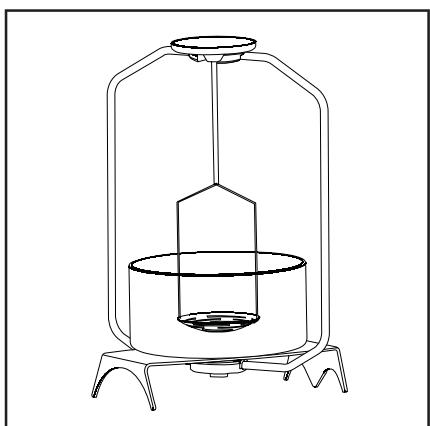
To determine the specific gravity of solids when their density is greater than that of the liquid in which the sample is immersed, use:
