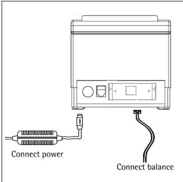
Check to make sure that the power switch of the printer is in the OFF position before connecting the printer according to the figure above.
