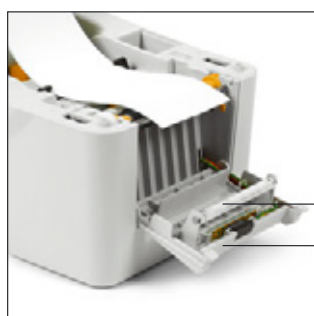
Peel-off roller Backing paper opening
