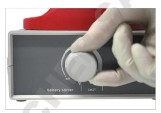
After completing the mixing procedure, switch off the magnetic stirrer, remove the sample holder from pluriPlix® and remove the reaction tubes from the sample holder.
