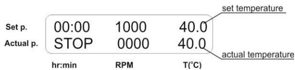
Fig.4 Control panel in operation mode
