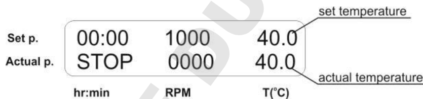
Fig.4 Control panel in operation mode
