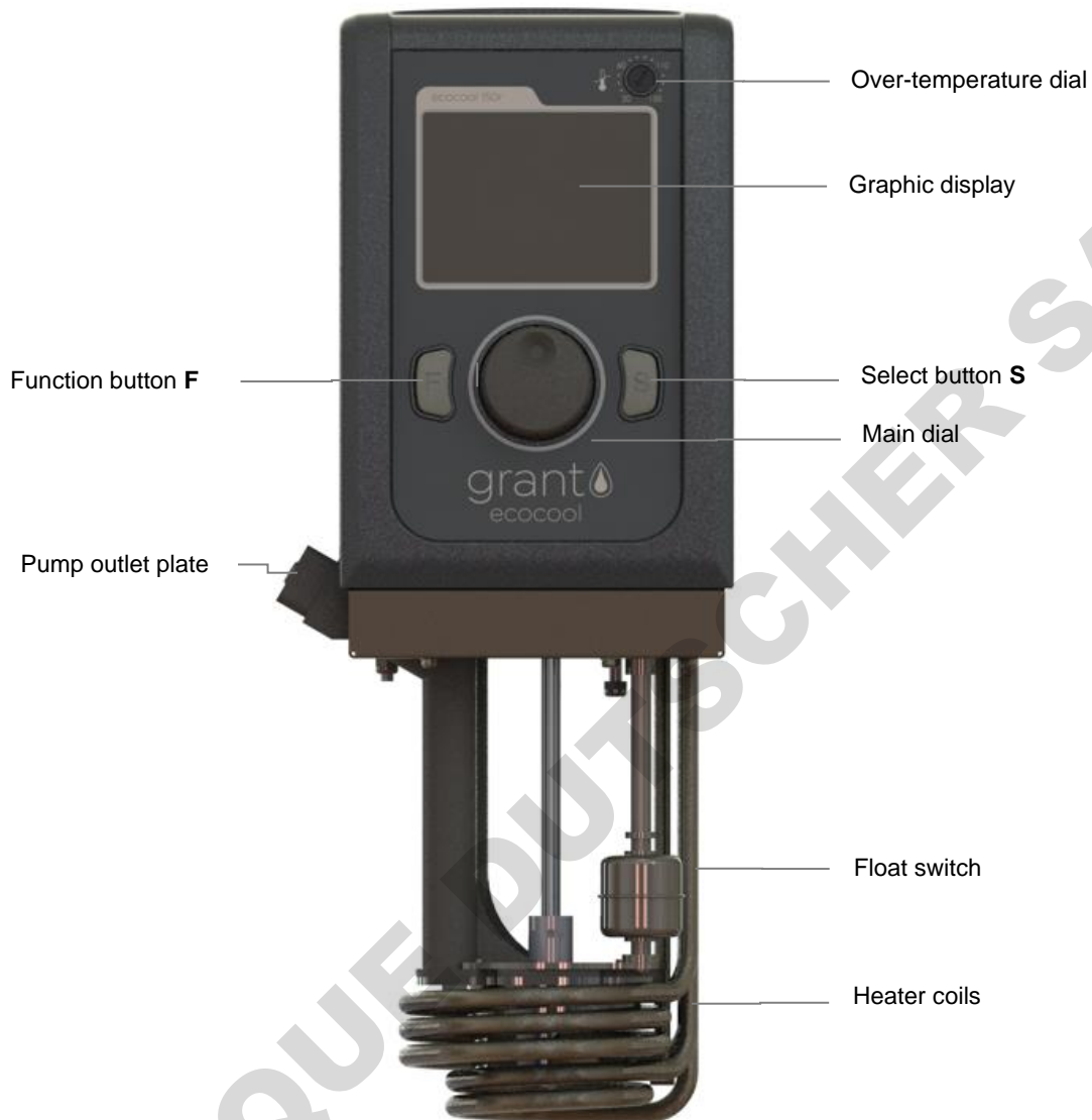
Figure 1: Heating circulator front panel
