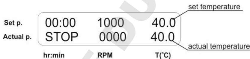
Fig.4 Control panel in operation mode
