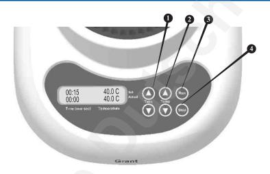
You can accurately set the temperature and time required for your specific task by utilising controls **1** and **2**.
