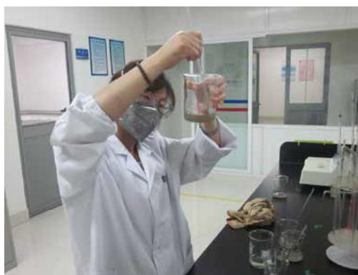
Fig 2. Addition of sample and HCl to a beaker.
