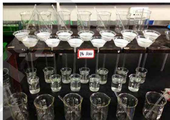
Fig 3. Retention of \text{PbSO}_4 precipitate using Whatman Grade 40 filter paper.
