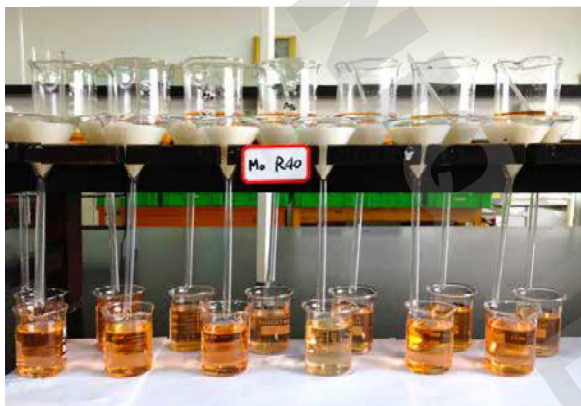
Fig 2. Retention of lead molybdate precipitate using Whatman Grade 40 filter paper.
