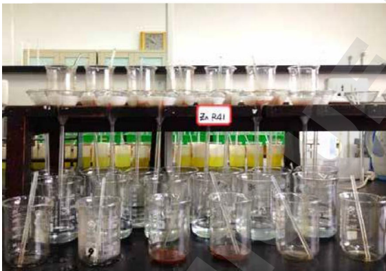
Fig 4. Use of Whatman Grade 41 filter paper in zinc analysis.
