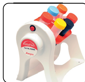
Change inserts to accommodate varying tube sizes
