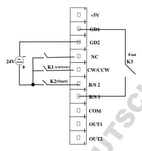
a. In pule mode, disconnect K2 after short connection, the motor start wroking. Disc onnect again after short connection, the motor stop working.
