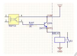
If connect with relays, when the motor running, K1 connect; when the motor stop running, the K1 disconnect.
