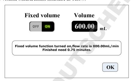
After turn on this function, the peristaltic pump will measure the volume automatically, when the volume reach set up volume, the pump will stop working automatically. The flow rate can be changed during the pump working.
