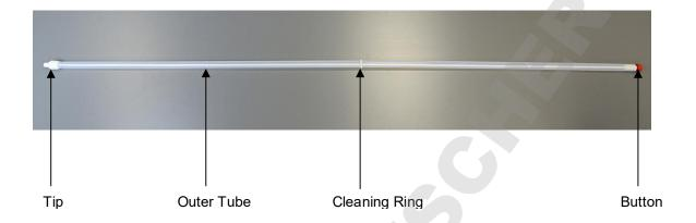
Diameter of Outer Tube: 25mm
