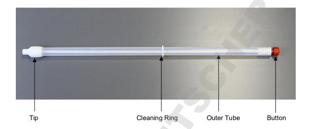
Diameter of Outer Tube: 25mm
