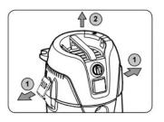
Put the upper part of the motor back in the tank and secure it with the latches.
