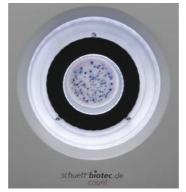
Various coloured colonies on filter disk with adapter for Petri dishes with Ø 50-60 mm.
