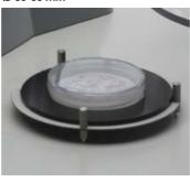
For central positioning of Petri dishes up to Ø 60 mm.
