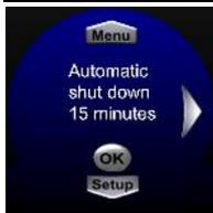
Choose the time after which the device automatically switches off, if it is not operated.
