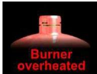
The schuett phoenix II is suitable for continuous operation (120 min) at fully opened gas and air supply, the burner may not overheat. However, if the burner gets too hot due to inappropriate conditions such as back reflections of heat or unfavourable setting of flame, the device automatically switches off. The remark “Burner overheated” is shown in the display.
