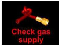
In case during automatic (re-)ignition the burner may not produce a flame after 10 seconds, the schuett phoenix II automatically and permanently shuts the gas supply. The display shows “Check gas supply“. See “Troubleshooting”, page 32.
