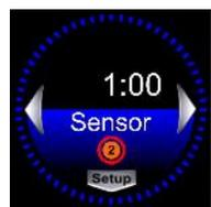
Activate the burner in sensor mode by moving quickly in front of the sensor.
