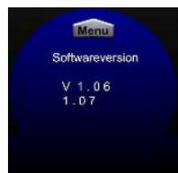
In case of a defect of the burner, please mention the two version numbers stated in this setup level.
