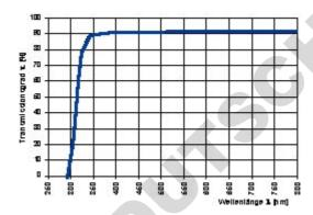
Between 0.15 und 0.40 mm glass thicknesses, the light transmittance is  $\tau_{VA} = 91.8\%$ . In the visible range of the spectrum D 263 M is without absorption. The excellent UV absorption properties makes D 263 M an ideal material for use in fluorescence microscopy.
